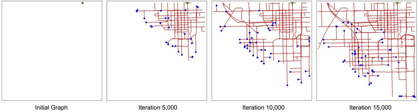
Figure 3: We visualize the partially constructed graph  $G$  (red) and the active vertices queue  $Q$  (blue) from different iterations in the construction procedure. In this example, the algorithm begins with a single vertex (green) at the upper-right corner of the region.
