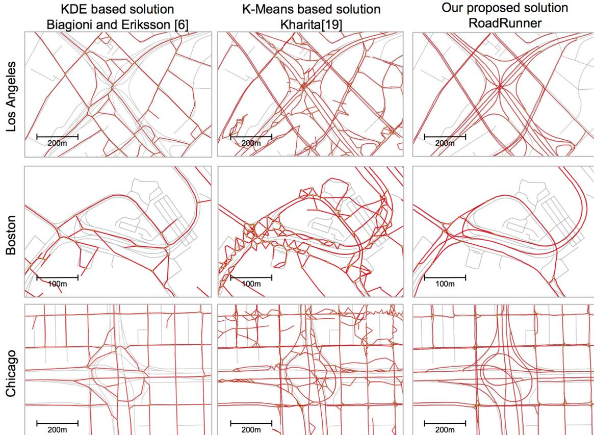
**Figure 1: Motivation.** GPS-trajectory based mapmaking algorithms running on complex interchanges in major cities. Red lines show algorithm output overlaid on underlying ground truth map in gray. Two existing algorithms are on left, our proposed RoadRunner algorithm is on right. Both existing approaches connect parallel segments on highways, often with many small, spurious crossing segments, and also add incorrect intersections where roads of different heights cross.
